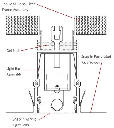
Section View at Interior Grid with Light Bar Assembly
