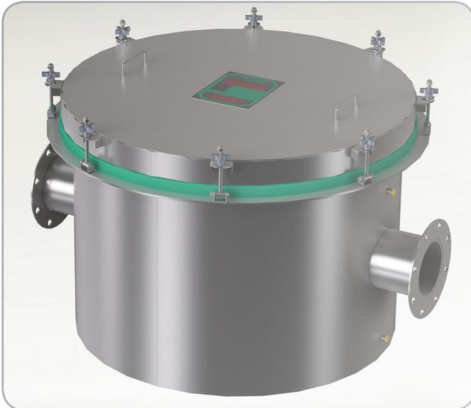
Camfil CamContain FB-R and GB-R Housings are designed for use in critical processes where hazardous airborne materials must be prevented from escaping to the atmosphere. Air filters may be replaced from the topside of the unit using a control barrier to protect change-out personnel from contaminants within the housing or captured by the filters. The unit may be mounted vertically or horizontally.
