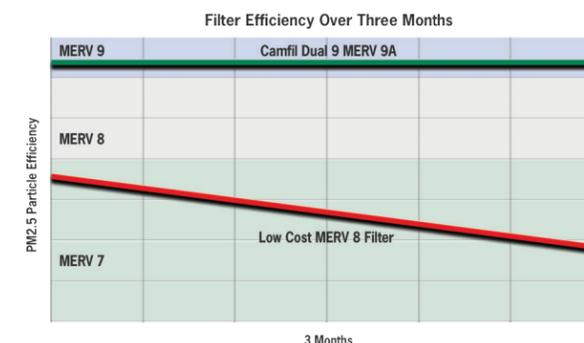
Area between the efficiency lines reflects particulate passing through the filter, collecting on secondary filters, heating and cooling coils, all which hinder total ventilation operating efficiency.
