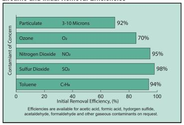
Camfil's unique molecular filtration testing laboratory runs tests according to the following standards: ASHRAE 145.1, ASHRAE 145.2, ISO 10121-1 and ISO 10121-2. The initial removal efficiencies referenced in the chart above were determined by challenging full size (24" x 24") filters with realistic gas concentrations in 2,000 CFM of air at 50% RH and 72F. More information on this unique testing facility can be provided.
