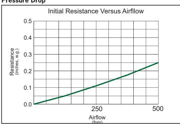
(Schedule air filters for change when initial pressure drop has doubled.) Final pressure drop should not exceed 1.5" w.g.
